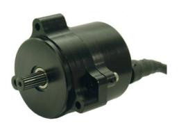
Permanent magnet alternators can tolerate high ambient temperatures and vibration allowing them to be directly mounted to racing engines. The separate regulator can be mounted in a location where the temperatures and vibration levels are lower. When used together with the DC2 "Buck" regulator, the alternator provides high current, at stable voltage, over a large range of rotation speeds from a very small and lightweight package.
